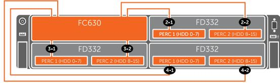
Diagrammatic representation of controller enumeration for split single host mapping configuration.
